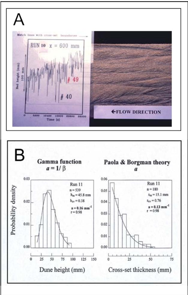
**Figure S2.** A) Time variation in bed elevation at a point controlling the vertical sequence of cross-set thicknesses. The same principle applies without sediment aggradation. B) Distribution of experimental dune heights and cross-set thicknesses from Leclair (2000), with respective functional parameter ' $a$ ' illustrating the Paola-Borgman theory (1991).
