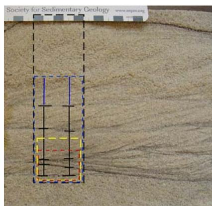
**Figure S5.** Illustration of the various cross-set distributions considered in an at-a-point vertical section in a partially (or completely) preserved coset. Examples from Run 10 (Leclair, 2002).
